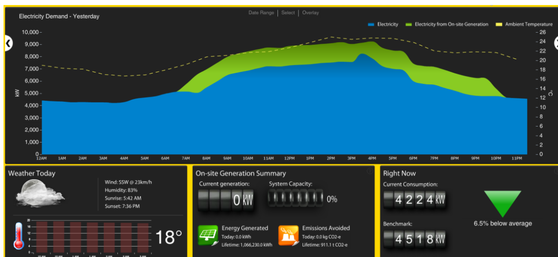
Picture 1 – Example dashboard of a Real-Time Energy Monitoring Solution
